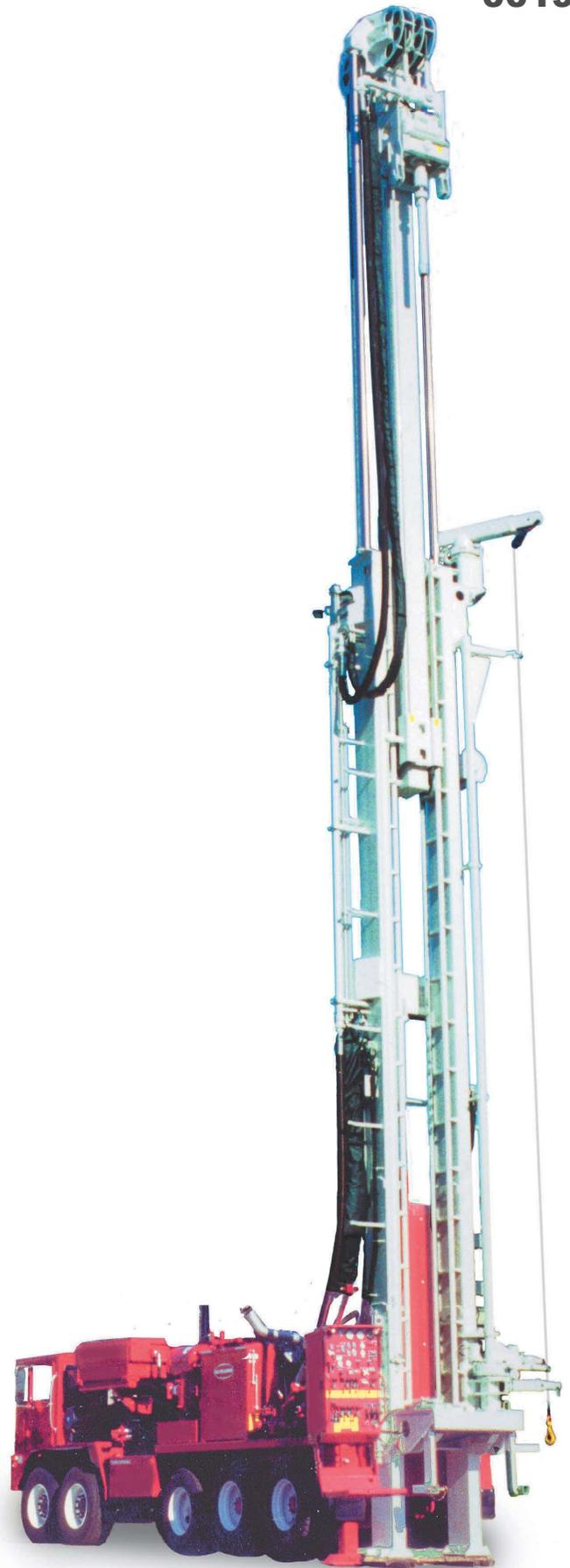
**CARRIER MOUNTED RIG EQUIPPED WITH TELEMAST**
