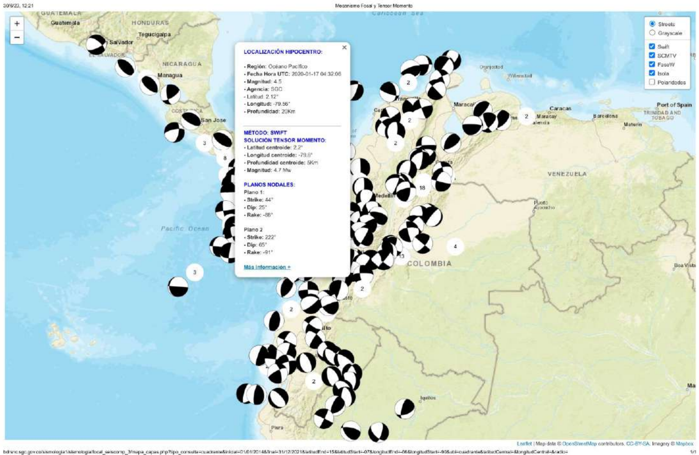
Figure 1. Focal mechanisms calculated by the SGC of earthquakes occurred between 2014 and 2021. From each focal mechanism, the user can access the detail of the moment tensor solutions for each earthquake
