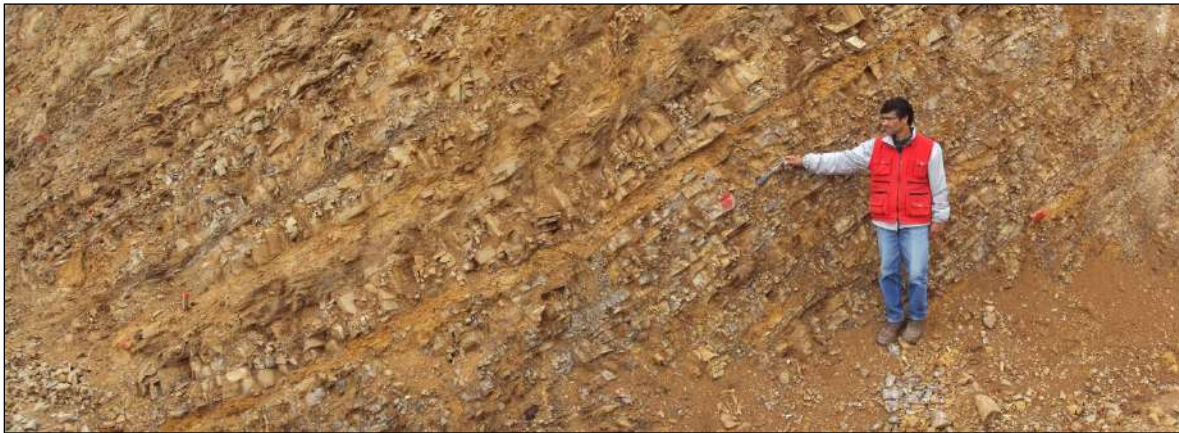
Figure 9. Porcellanites with some intercalations of claystone in lentiform beds; the rock is weathered and takes on a yellowish coloration.
